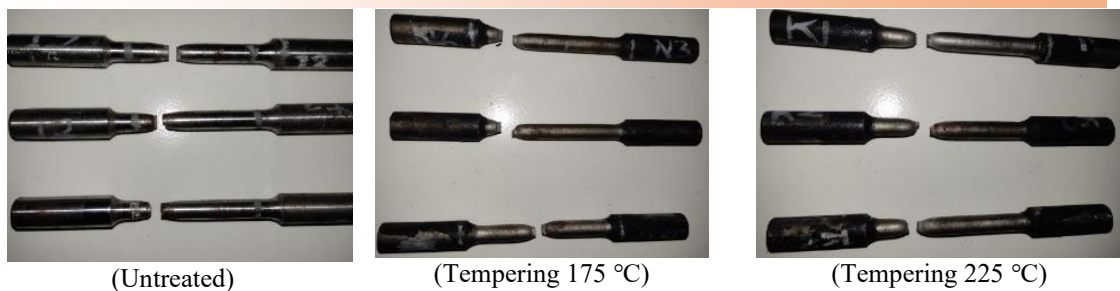
Fig. 5. Specimen fracture results after tensile testing
