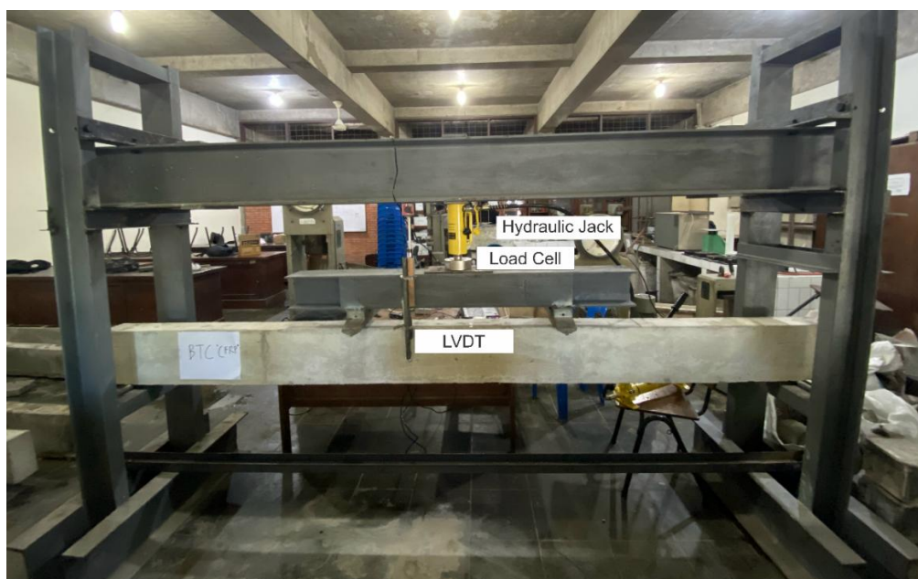
Figure 5. Setup flexural test in Laboratory of HKBP Nommensen University
