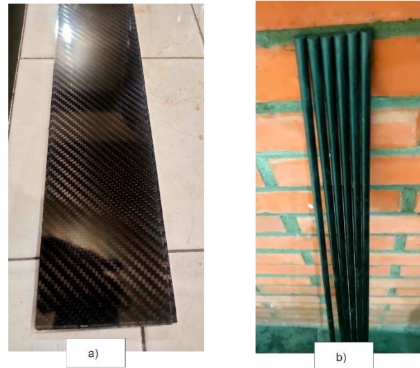
Figure 3. a) Carbon fiber sheet and b) rod rebar Carbon Fiber
