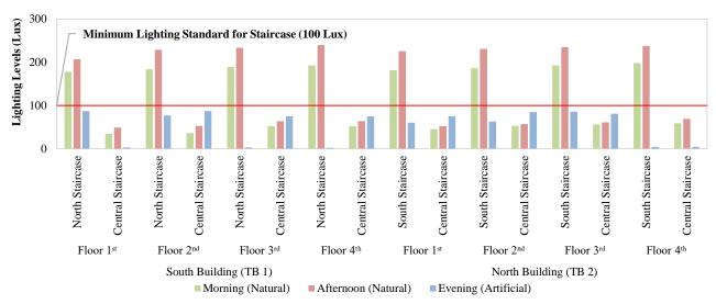
Figure 15. Diagram of lighting levels in the staircases.
