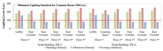
**Figure 11.** Diagram of lighting levels in the east side common rooms.
