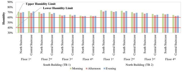
Figure 23. Diagrams of humidity levels in the staircases buildings TB 1 and TB 2.
