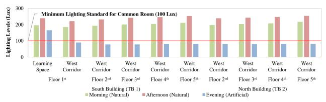
**Figure 12**. Diagram of lighting levels in the west side common rooms.
