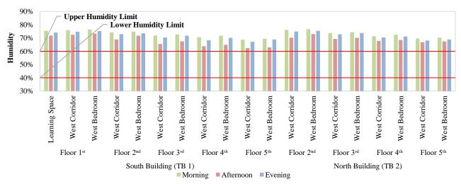
Figure 22. Diagram of humidity levels in the west side buildings TB 1 and TB 2.
