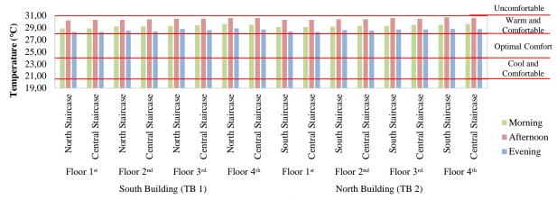
**Figure 19.** Diagrams of air temperature levels in the staircases buildings TB 1 and TB 2.
