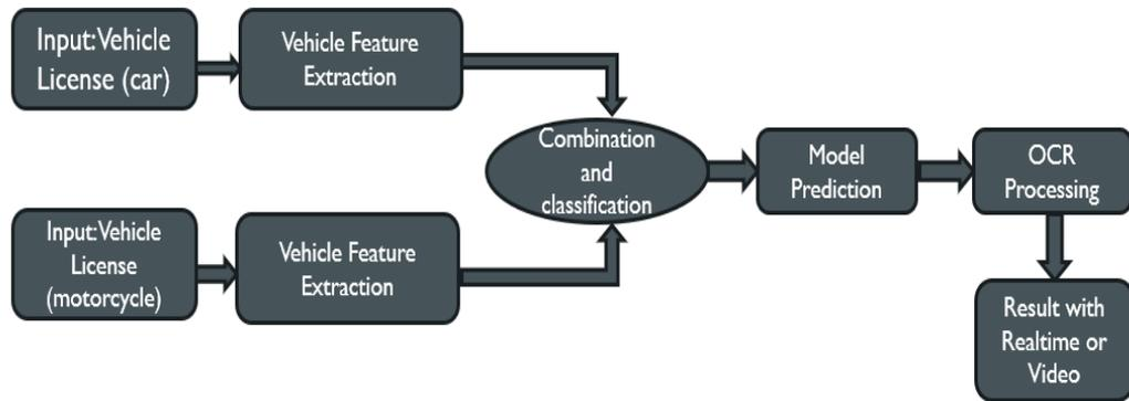
Figure 1. Block Diagram Detection of Indonesian Vehicle License Plates
