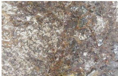
Figure 5. E 6013 Seawater Electrode Day 15
