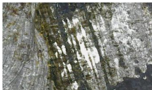
Figure 8. E7018 Rainwater Electrode Day 15
