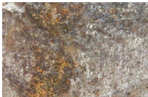
Figure 7. E 7018 Seawater Electrode Day 15
