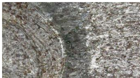
Figure 4. E6010 Electrode Rainwater Day 15
