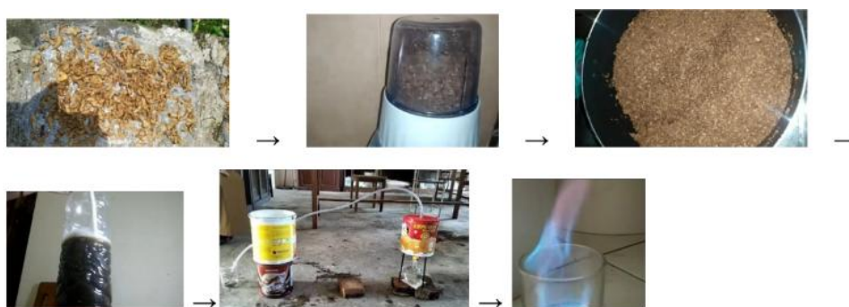
Figure 5. Design of a simple bioethanol production tool from potato peel waste
